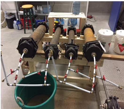
Figure 9: Chlorination Pilot Testing Pipes
