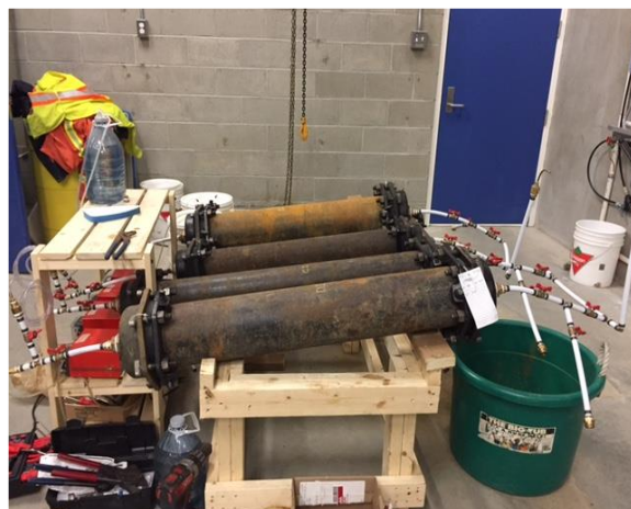
Figure 10: Chlorination Pilot Testing Pipes
