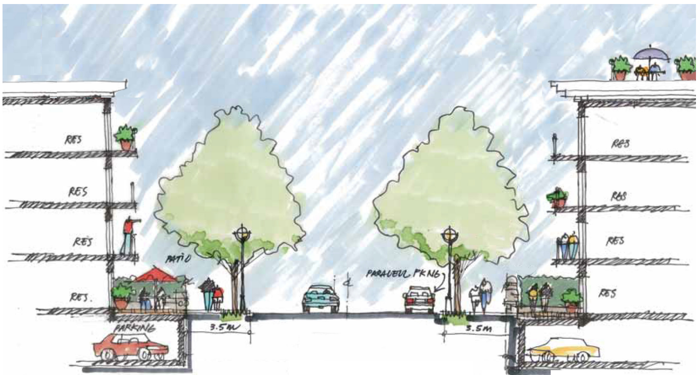
This section shows 4-storey residential apartments. Entrances are level with the sidewalk and ground floor units are ground-oriented with semi-private patio spaces defined by low shrubs and low fences. Residential parking is provided underground. Shared rooftop amenity spaces and balconies are encouraged.
