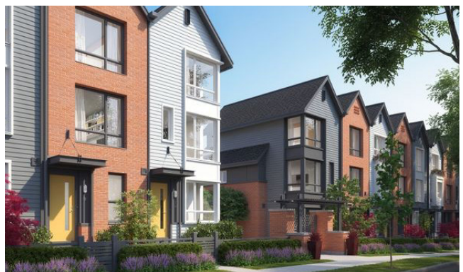
Guidelines c and l: Varied materials and colours on each townhouse provides distinct character and rhythm along the street, pitched roofs and landscape contribute to the character, and blocks of townhouses are limited to eight
