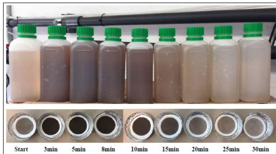
Images of Backwash water samples and Total Suspended Solids test results at different sampling times.
