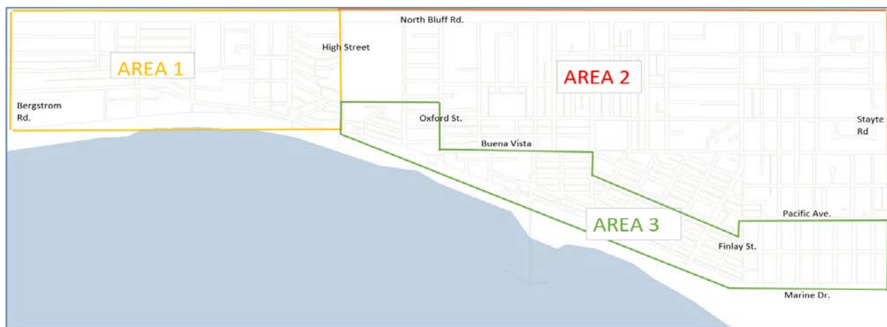
Figure-5, Unidirectional Flushing Areas 1, 2 & 3
