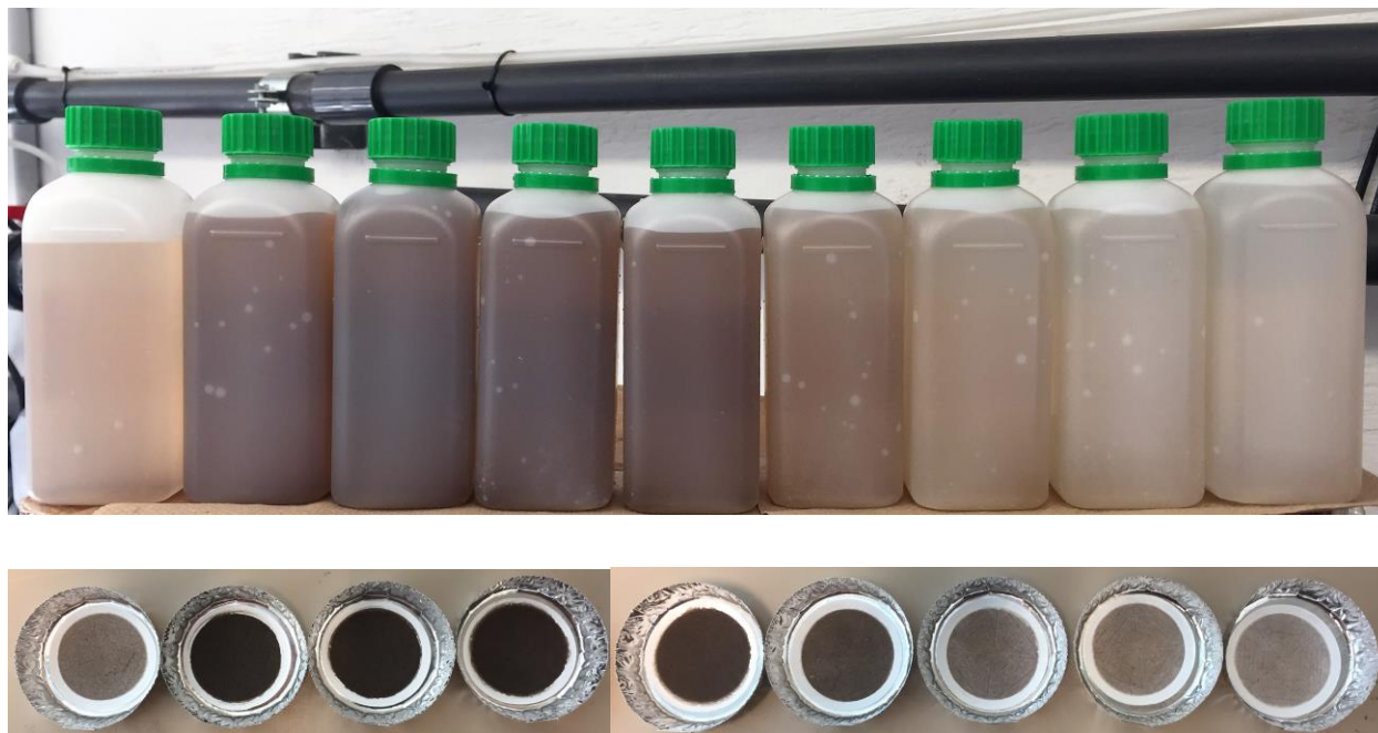
Start 3min 5min 8min 10min 15min 20min 25min 30min Figure 2.20 Backwash water samples and Total Suspended Solids test results at different times, after ozonation study.
