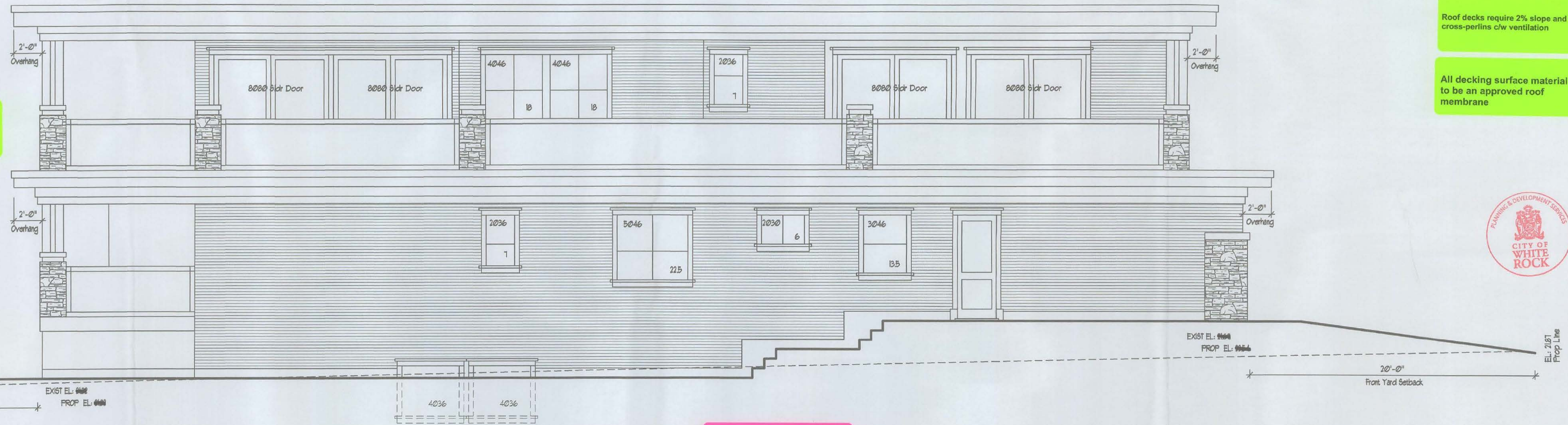
LEFT ELEVATION SCALE 1/4" = 1'-0" SPATIAL SEPERATION CALCULATIONS WALL AREA 1610 SQFT LIMITING DISTANCE 4'-0" (1.2 m) MAX ALLOWABLE UNPROTECTED OPENINGS AT 7% = 116 SQFT PROPOSED UNPROTECTED OPENINGS = 92 SQFT
