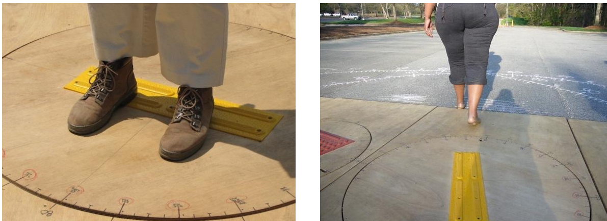
(a) Bars perpendicular to intended travel direction (b) Bars parallel to intended travel direction
